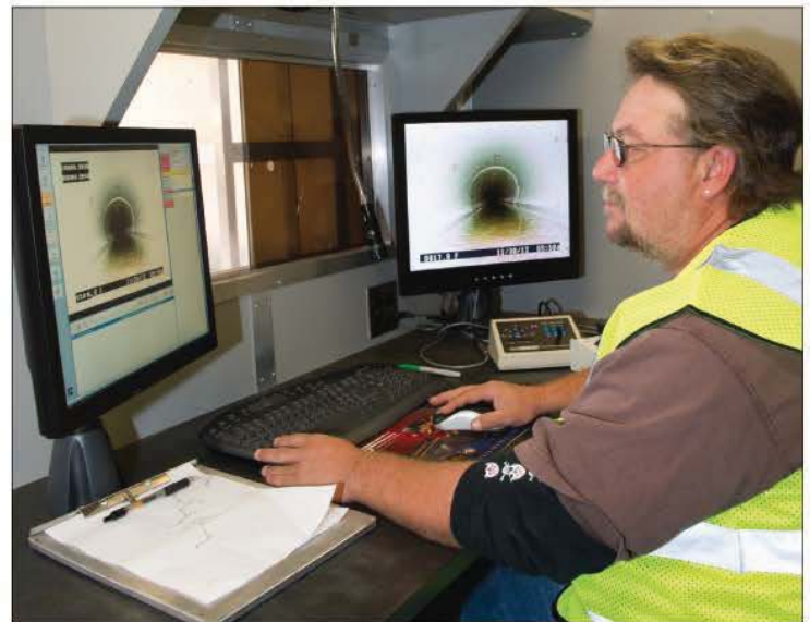
Leroy Thornton looks at a closed-circuit-video feed of a sewer line from inside the Aries CCTV truck.
